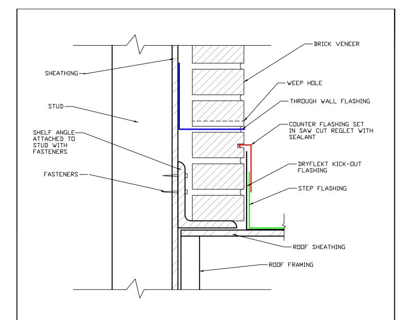
NOTE: The kickout flashing shall be min. 4" x 4" in. As required by IRC code R905.2.8.3 and be angled between 100° -110° to deflect water from dumping behind the siding and the end of the roof intersection.
